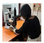
Camera with Adapter: Attached to microscopes, the camera allows for capturing images and recording videos, which can be used for analysis, presentations, and documentation of experimental observations.
