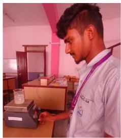
**Dip Coating Unit ("Holmark")**: Enables thin-film deposition on substrates, critical in materials science and nanotechnology research within electronics, especially for sensor and coating applications.
